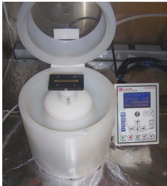
Figure M2b.2. Spin coater being used to cast thin films of the binder on a Zn-Se FTIR window.
